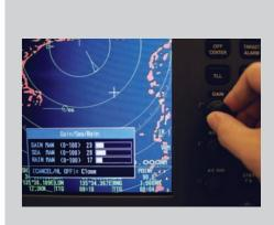
Featuring dedicated rotary knobs to adjust GAIN/STC/FTC for straightforward operation
